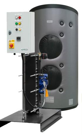
The Adveco PPS is a range of packaged plate heat exchanger systems from 100 to 600 kW designed to operate with a stainless steel buffer vessel to provide a high-capacity source of domestic hot water to a building.
